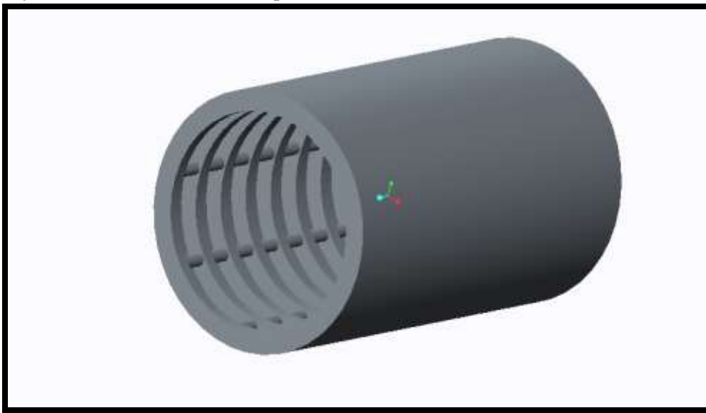
Figure 3. 3D Model of sandwich beam (semi monocoque)
